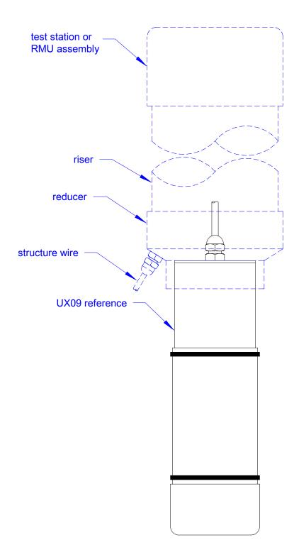
Typical installation of Model UX09 reference electrode on an RMU or test station riser. Components shown in dashed lines are user supplied.
