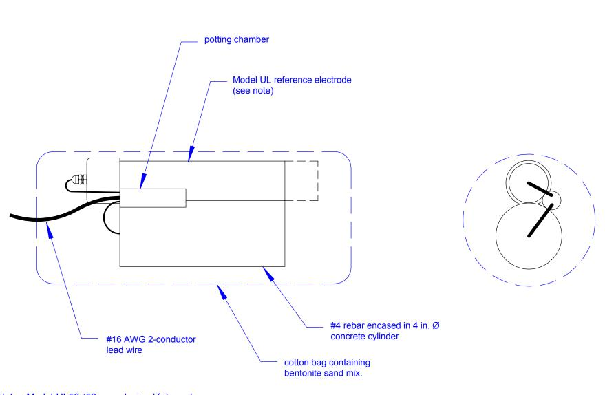
Note: Model UL50 (50 year design life) can be substituted for the Model UL. This will extend the electode length as shown by the dashed line. The model designation for the extended life reference is Model UX15A-xxx-LWnnn.
