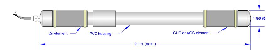
Model UDH is limited to a maximum service temperature of 200°F. When it is used beneath a storage tank containing heated product, it should be buried deep enough so that the temperature at the electrode is less than 200°F.
