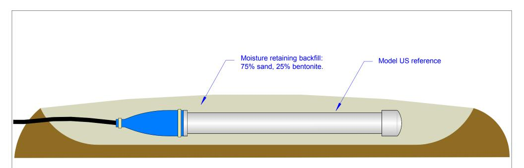
When installing a Model US reference electrode in a horizontal position, best performance will result if the electrode is placed in a small cavity in the soil. Once the electrode is positioned, cover it with at least an inch of a moisture retaining backfill. Thoroughly wet the backfill with potable water. Measure and record the potential using a recently calibrated portable reference electrode.
