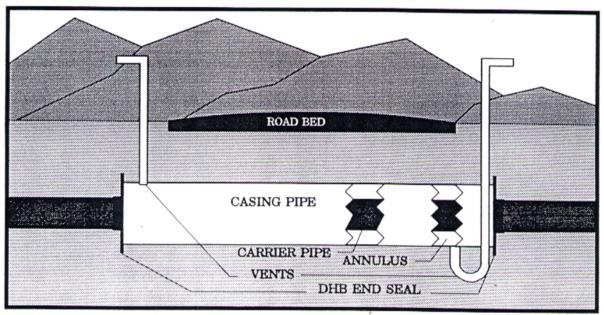
There is no "messy" cleanup when the job is complete or if the casing is ever removed. There is no possibility for toxics to leach into the surrounding soil. The process is designed to quickly and accurately fill the annular space with the proper amount of material. In addition to these benefits, this product and the process offers substantial cost savings compared to alternative casing fillers currently available.
